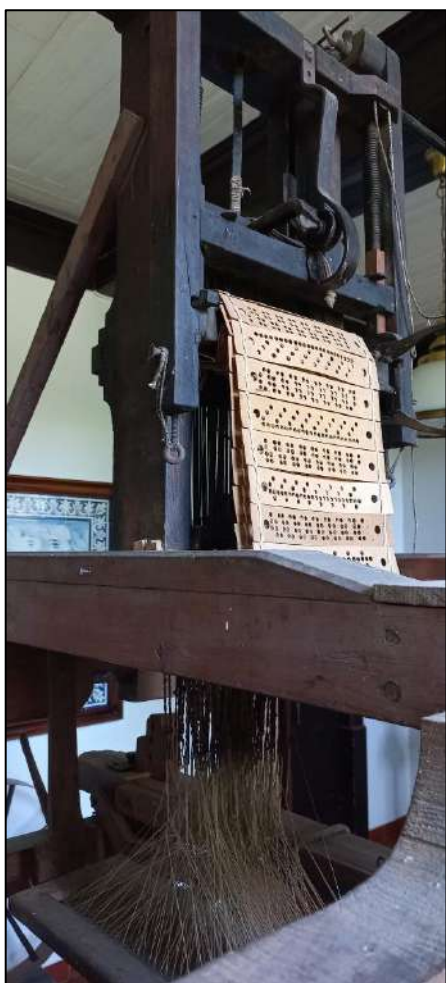
Fig. 14. Tear Jacquard. Fabrica Ceppas,
